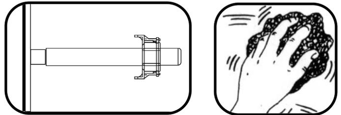
1. For installing a Hex Nut Insert with a Stick-On, simply attach the appropriately sized Tap-On to the Hex Nut Insert. Clean the mounting surface with steel wool and alcohol.
