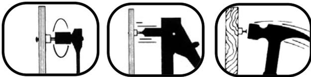
1. For installing a Hex Nut Insert with a Tap-On, it will be necessary to drill small holes in the form at the locations where inserts are desired. Measure and mark the form wherever an insert is needed and drill a 3/16" hole. Then, simply bolt, rivet, or nail the tap-on to the form.
