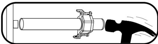
2. Tap Hex Nut Insert or regular insert gently on to the tap-on. (Never hit the Insert hard and always wear safety glasses.)
