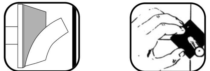
2. Peel the white backing off then press the Stick-On firmly in place using the corners of the Stick-On to align for critical placement.
