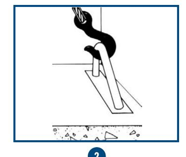
Measure and mark the form where Pulling Irons are needed and cut a 1.5" x 7" slot. Set up and oil form before installing Pulling Irons. This keeps the part free of oil and grease. Insert Pulling Iron into slot in form so that the shielding plate on the Pulling Iron covers the slot. This prevents slurry from leaking through the slot.
