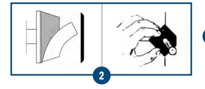
Peel the white backing off then press the Stick-On firmly in place using the corners of the Stick-On to align for critical placement.
