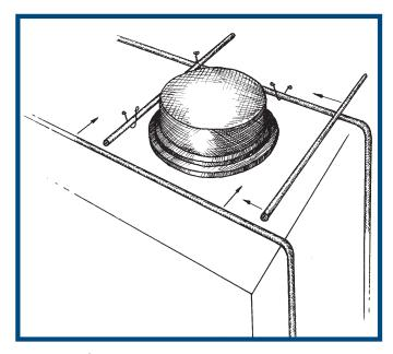
Put on the form and wire or caulk in place. Dimensions: 12.5" diameter x 4" deep. (o.d. = 15" diameter x 4.5" deep).
